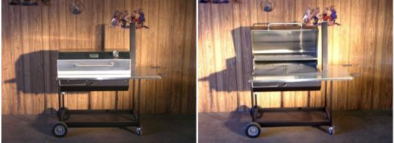
The New 20x36 Square Grill w/SS Hood Total Length including handles 48 inches Top of stack is 58 inches/ 32" Depth including wheels. Full Log Rack 20 inches by 36 inches long. Main cooking area has 2 piece meat racks framed in steel angles for strength, & removable 1/2 Shelf. All New Steel on Square Pits is 12 gauge for the Grills, 3/16" on the fireboxes, & 14 gauge on the SS.
