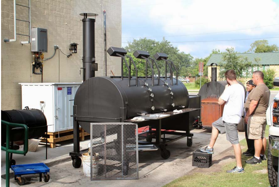
42" diameter by 10 foot Main Chamber, Three Door with 42" x 42" Firebox
