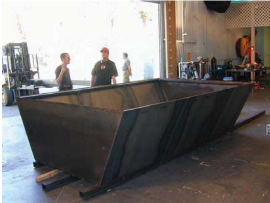
4 foot by 8 foot main steel box
