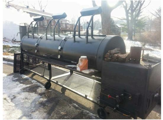
30" diameter by 10 ft Main Chamber, Three Door with 30x30" Firebox. I recommend Two Door
