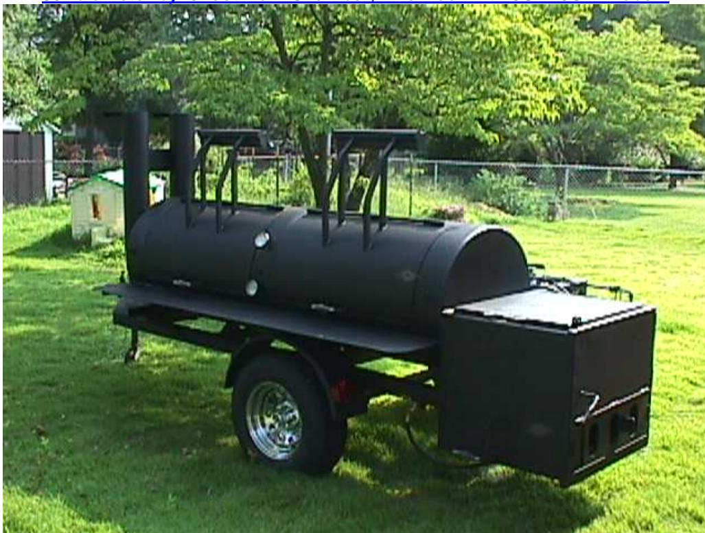
THE 30" x 8 foot Main Chamber- Tandem Axles-Old Style with Single 6K Axle Trailer 4-1/2' Wide by 15ft Long. 2ft wider with log rack option. 30" diameter by 8 foot Main Chamber, Two Door with 30"x 30" Firebox.
