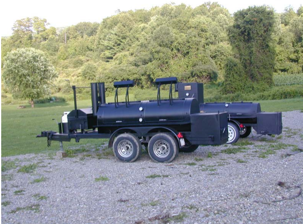
THE 30" x 8 foot Main Chamber- Tandem Axles-Fold up Fish Fryer Table Trailer 4-1/2' Wide by 15ft Long. 2ft wider with log rack option. 30" diameter by 8 foot Main Chamber, Two Door with 30"x 30" Firebox.
