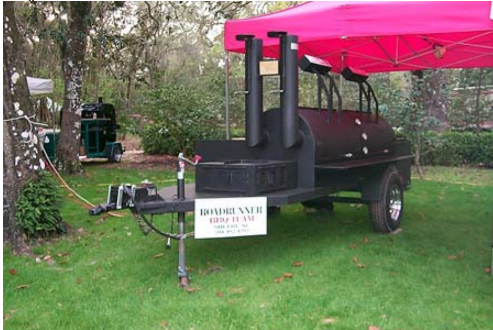
THE 30" x 8 foot Main Chamber- Tandem Axles-Old Style with Single 6K Axle Trailer 4-1/2' Wide by 15ft Long. 2ft wider with log rack option. 30" diameter by 8 foot Main Chamber, Two Door with 30"x 30" Firebox.
