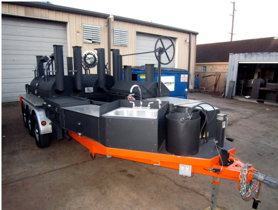
Dual 36" x8ft Smokers & 3 Row Pullout Shelves. Capacity 72sq ft per Smoker
