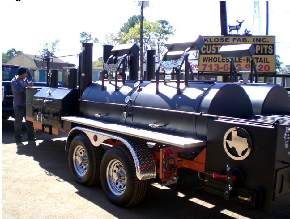
Dual 36" x8ft Smokers & 3 Row Pullout Shelves. Capacity 72sq ft per Smoker
