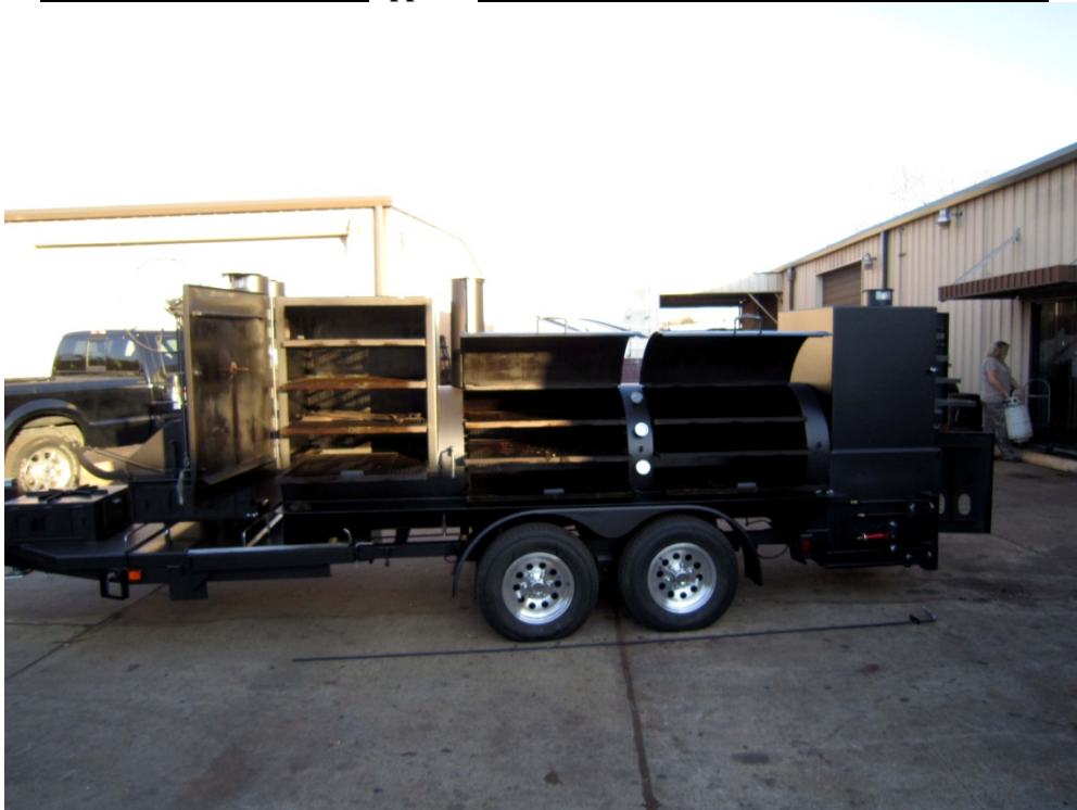
"ROCK'S RESTAURANTEER & CATERING WAGON" CHECK OUT THE EXTRA WIDE 30" X 48" STEAK GRILL & WARMING OVEN The 36" X 8' with Upright-Approx. Capacity 102 Sq. Ft. & Feeds about 1200-1350
