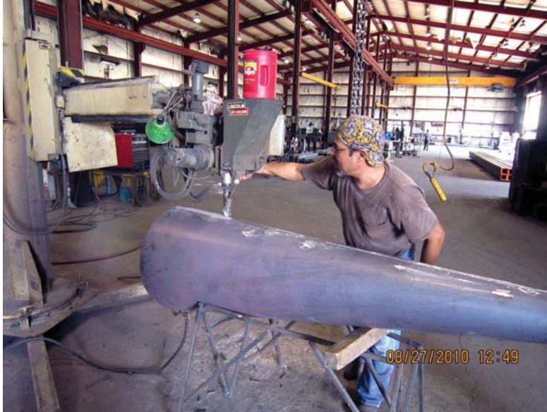
Submerge Arc welding the reducers for the rear assembly's
