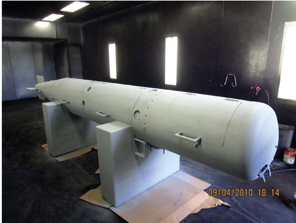
Automotive Base Primer Coats Completed
