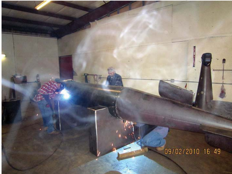
Rolling Base Stands welded on/Notice electrolysis effect from welding
