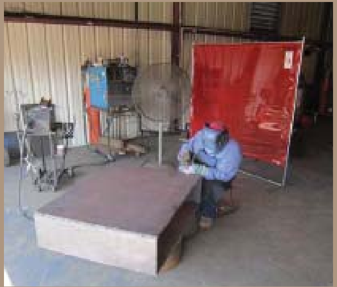
THE BASE STANDS WITH 8" WHEELS RECESSED WEIGH 1000 # EACH.
